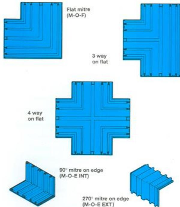
Factory welded intersections are available for Supercast Angleguard
