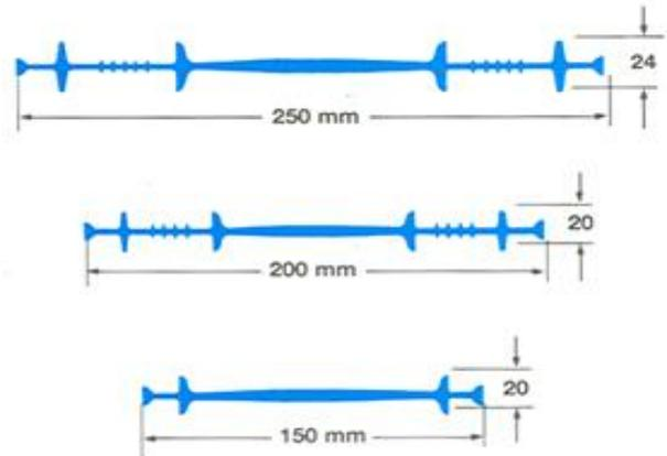
All centrally placed Supercast waterstops incorporate an eyeletted, reinforced edge flange. This enables them to be easily positioned by wiring to surrounding reinforcement.
