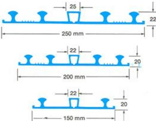
All Rearguard sections incorporate a nailing flange with a reinforced edge to provide a secure fixing that will resist tearing.
