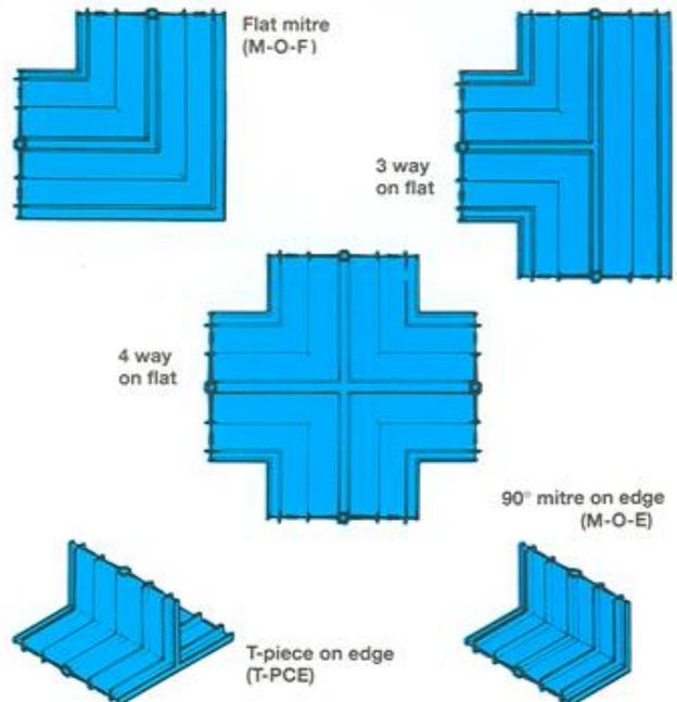
Moulded Supercast Rearguard R to Watafoil and Rearguard R to XHD Watafoil
